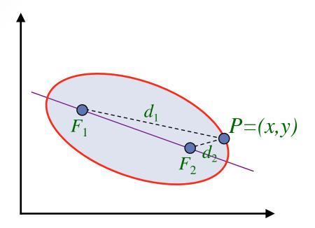
• The sum of the two distances d<sub>1</sub> and d<sub>2</sub>, between the fixed positions F<sub>1</sub> and F<sub>2</sub> (called the foci of the ellipse) to any point P on the ellipse, is the same value, i.e.
