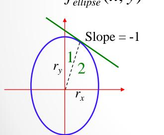
$$Slope = \frac{dy}{dx} = -\frac{2r_y^2 x}{2r_x^2 y}$$
